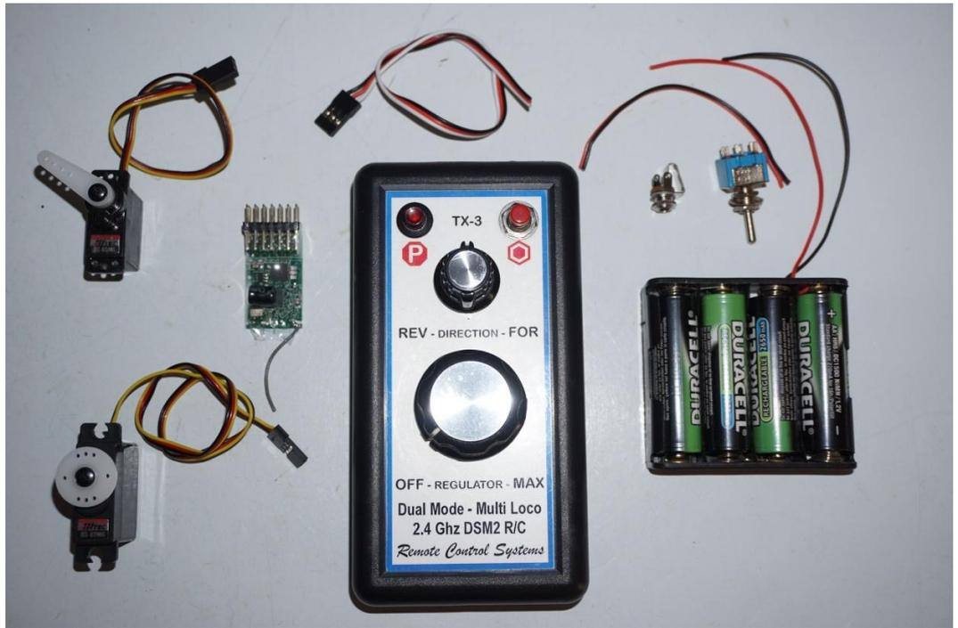
transmitter are using the AA batteries for scale. Both the HT-65MG and HT-82MG servos are on the left. The size difference is minimal, but could be critical depending on the locomotive
